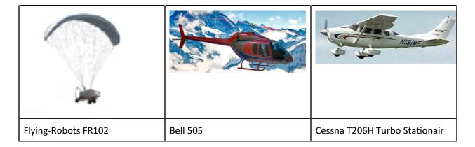
The soft-wing drone and the airplane are equipped with a piston engine, while the helicopter is equipped with a mono-turbine, this concept offering the best weight / power / reliability ratio in this power range.
